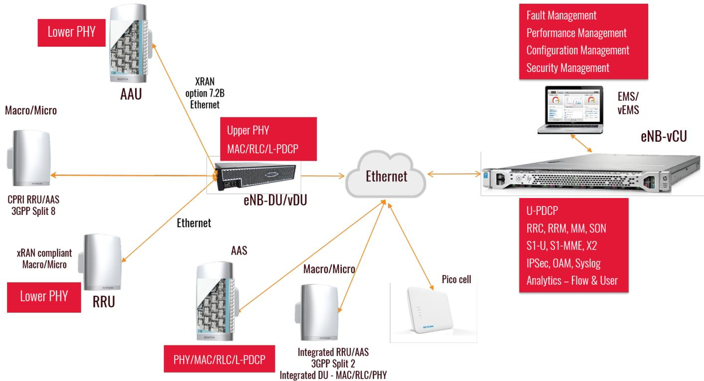
AltioStar has aligned its solution architecture nomenclature for its split eNB/gNB solution with 3GPP TR 38.801 in the following way
