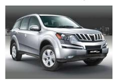
With the launch of its 'W4' model, 'Mahindra XUV500' - India's trendsetting SUV, now comes equipped with fuel-efficient micro hybrid technology. The technology automatically turns off the engine when idle or in neutral gear and restarts it once the clutch is pressed.
