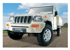
The new Bolero Pick-Up Flat Bed incorporates micro hybrid technology and is powered by Mahindra's trusted MDI Engine which delivers an excellent 13.86 kmpl with a load capacity of 1,250 kg.
